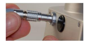
Connect the other end of the Volk Power Pass-Through Cable to the left side of the CLA housing at the connector marked:
