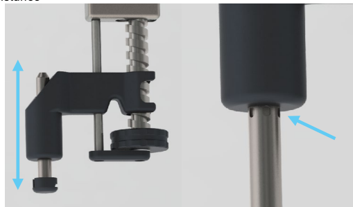
c) Check the free movement of the safety rod by sliding it up and down. When action is free the control marks will be visible
